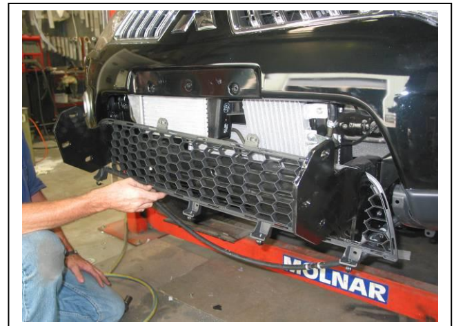
Figure 4: Grille fitment onto ECB steel mount brackets upon installation of mounts.
