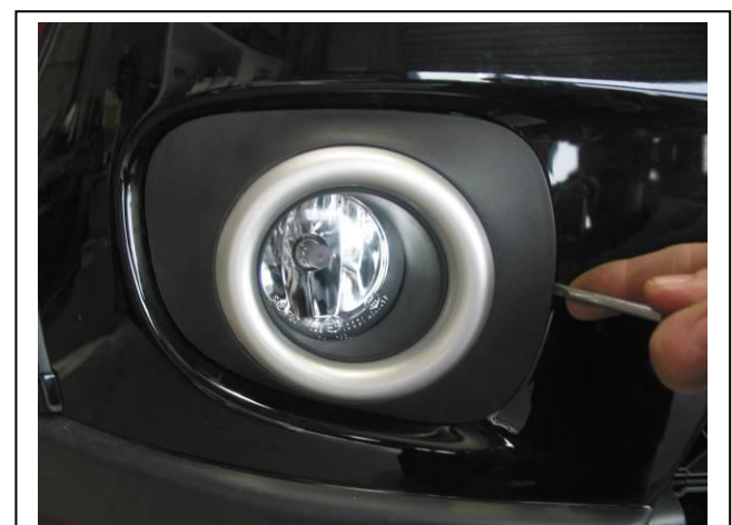
Figure 8: Use a flat bladed screw driver to carefully remove fog light covers.
